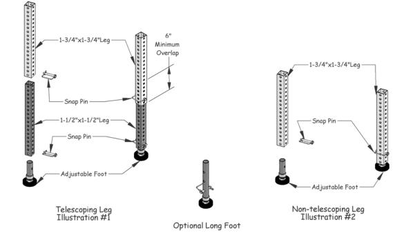
Assemble legs as shown either as illustration #1 or #2, the telescoping legs must not exceed the 6" minimum overlap.
